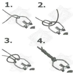
4. Attach wire hangers on each side of the frame 1/4 of the total height down from the top. Loop wire (not included) as illustrated to the left on the first hanger, and then repeat for the second hanger. Your frame is now ready for hanging.
